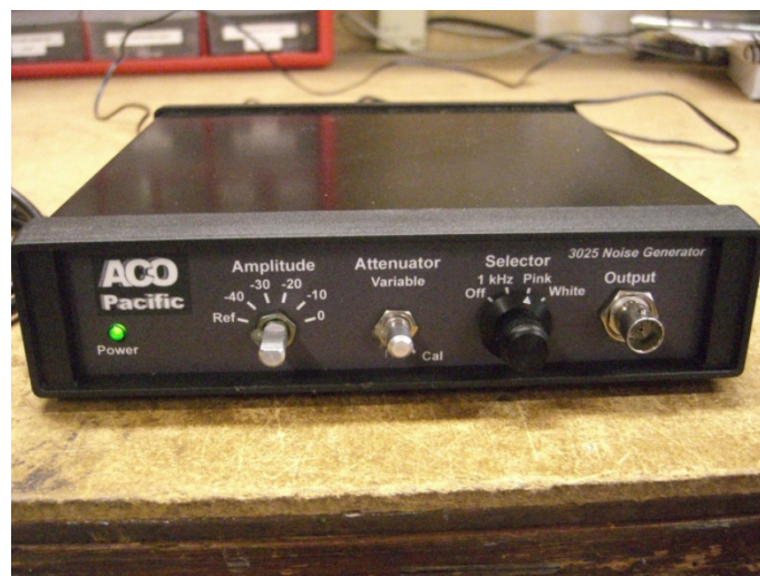
FIGURE 4 Noise generator selected for the OBSI calibrator
