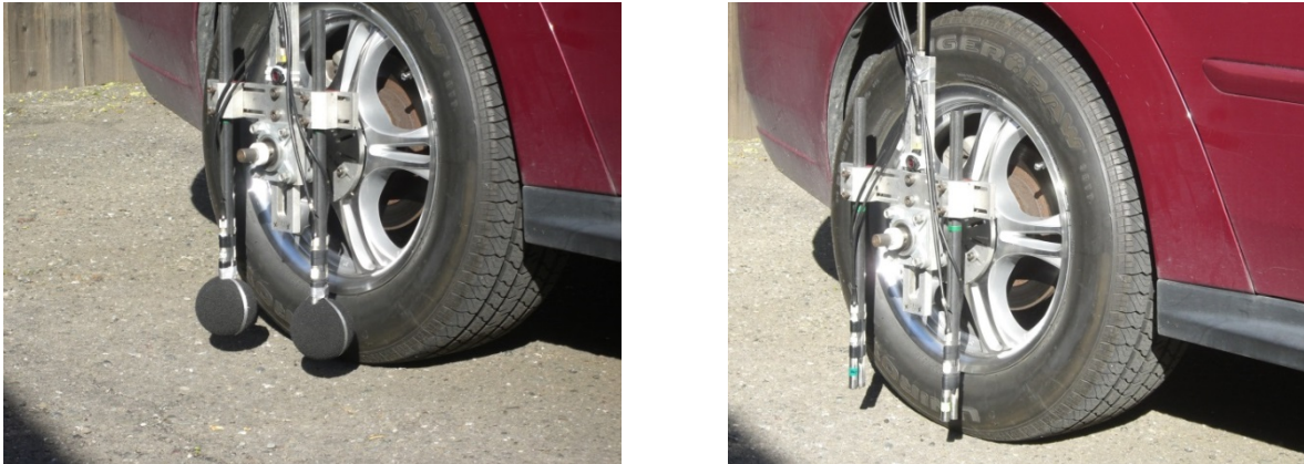
FIGURE 1 Sound intensity probe positioned for OBSI measurements with windscreens normally used (left) and without windscreen for illustration (right)
